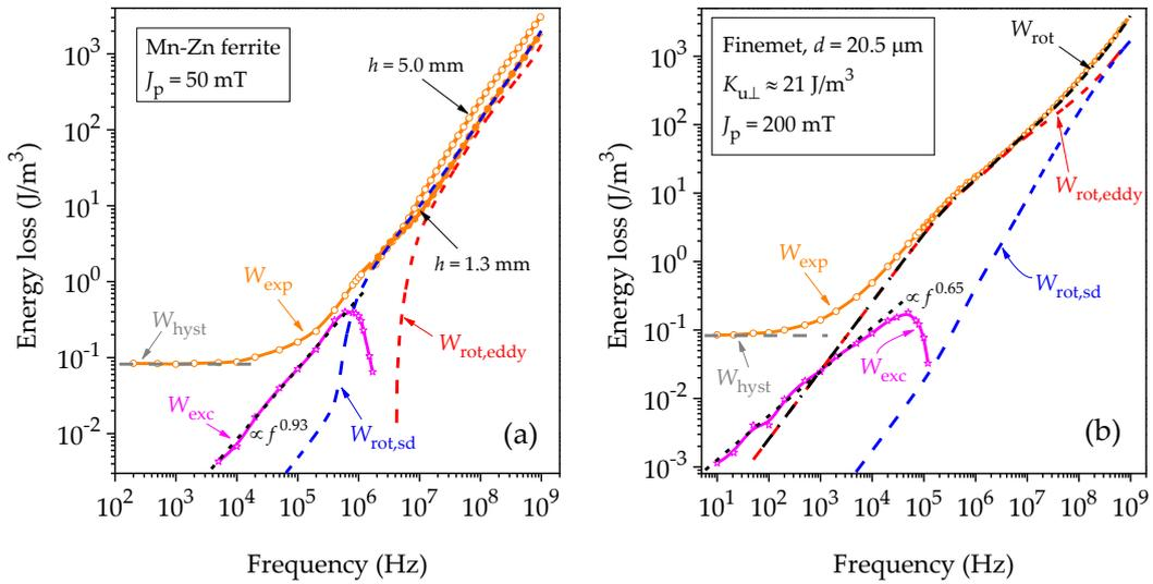
Figure 1: Broadband magnetic losses measured (a) in a Mn-Zn ferrite ring with two different values of thickness  $h$  and (b) in a 20.5  $\mu\text{m}$  thick tapewound nanocrystalline transverse anisotropy Finemet ribbon at a defined  $J_p$  level. The measured loss  $W_{\text{exp}}(f)$  is decomposed into the quasi-static hysteresis  $W_{\text{hyst}}$  component and the dynamic  $W_{\text{exc}}(f) + W_{\text{rot,eddy}}(f) + W_{\text{rot,sd}}(f)$  contribution.
